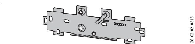
► Reposition the threaded stud on the mounting bracket (the stud has a self-tapping thread).
