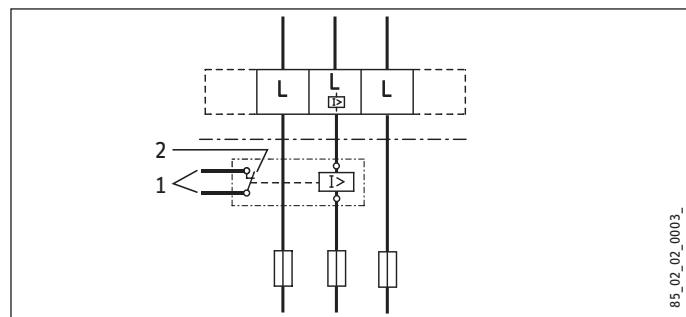
1 Control cable to the contactor of the second appliance (e.g. electric storage heater).
